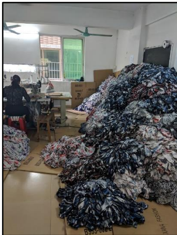
Semi-finished product stacked too high, on cardboard
